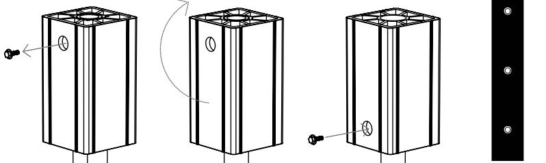
**3** **Wood Post** - Insert cable rail lag screws into wood post, and hand tighten using fitting as leverage.
