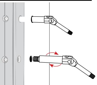
**5** **5A** - Install tensioning and non-tensioning cable rail fittings. Insert cable into non-tensioning fittings, run cable through intermediate posts.
