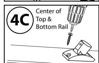
**4C - Install Intermediate Baluster.** Locate center of top and bottom rail. Using supplied hardware install intermediate baluster connectors on top of bottom rail and underside of top rail.
